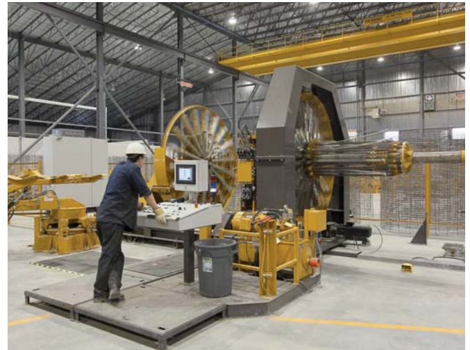
The HawkeyePedershaab CageFlex welding system at the new Lecuyer pipe plant automatically produces precision pipe cages using advanced weld technology that saves time and energy.
