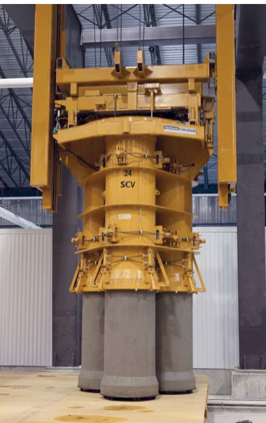
Here, a 24-inch Tri-Pac of RCP is demolded onto the moving floor of the HawkeyePedershaab pipe production system. Multi-form modules (1 to 4 molds per module) greatly accelerates production, allowing small bore pipes to be produced at a rate of less than a minute each.
