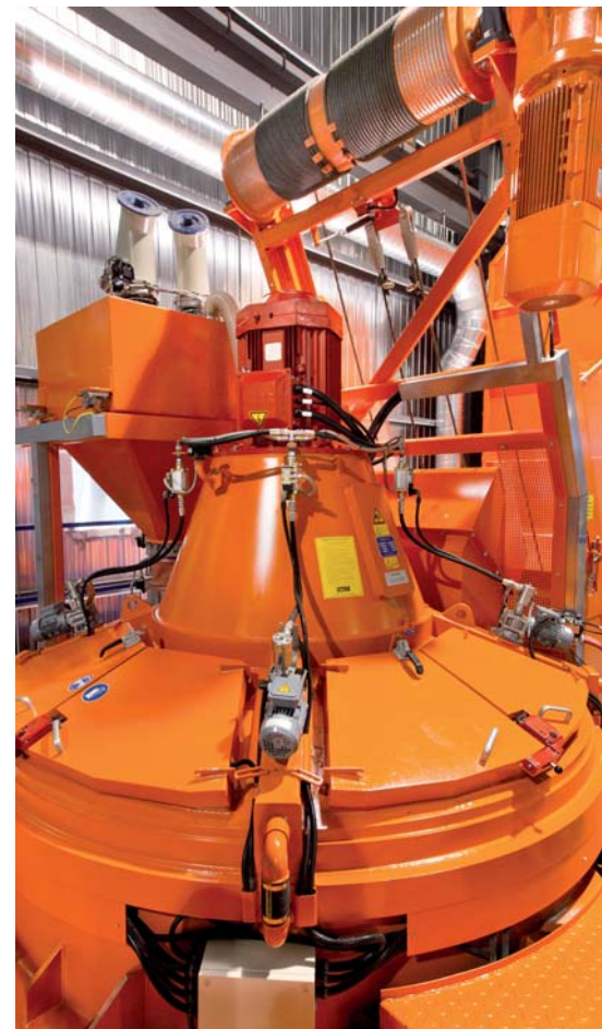
Even after three months of operations, the Wiggert HPGM 2250 counter-current planetary mixer at the heart of the ACT MobilMat batch plant looks clean enough to eat from. Automatic dust collection and mixer clean out systems help reduce maintenance and operating costs.
