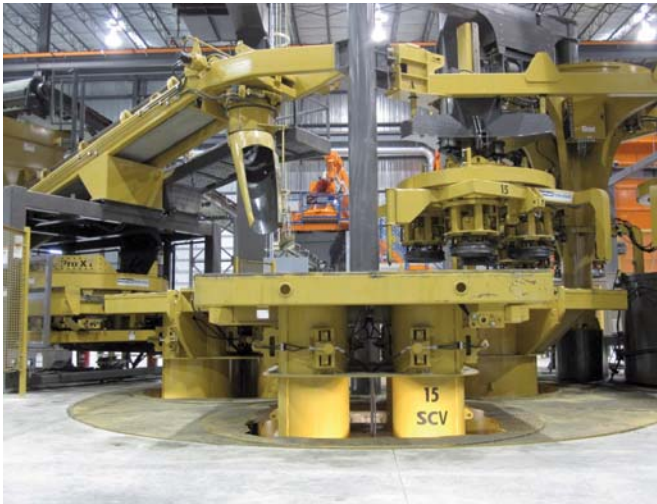
HawkeyePedershaab PipePro XT pipe production system installed in the new Lecuyer Group facility in Saint-Remi, Quebec, features unique turntable design that allows three sizes of pipe to be produced at the same time, providing flexibility and efficiency to meet varying market demands.
