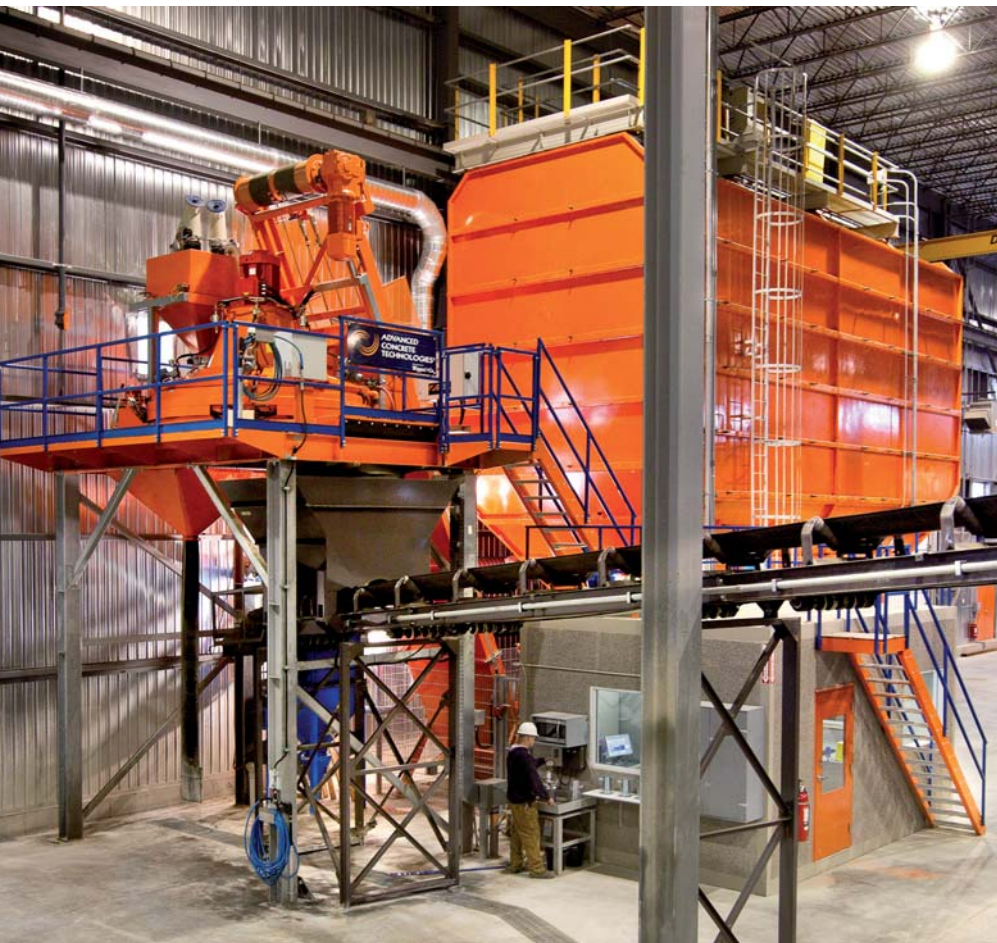
ACT MobilMat Mo80/4-PCS concrete batching plant is installed inside the new Lecuyer RCP plant to protect it from the weather. At left is the mixer platform containing a Wiggert HPGM 2250 high shear counter-current planetary mixer; four-compartment aggregate storage bins are to the right of the mixer. Precision dry cast mix is transferred to the HawkeyePedershaab pipe system via the overhead conveyor that extends from the mixer platform.
